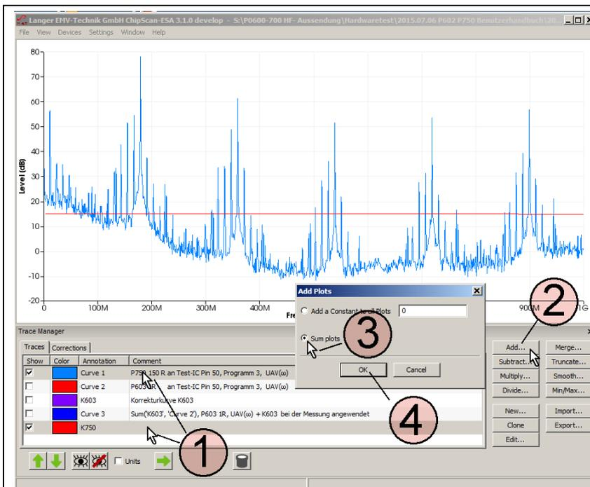
Figure 47: Correction after the measurement; performing the addition  $U_{IC} = U_{AV} + K750$
