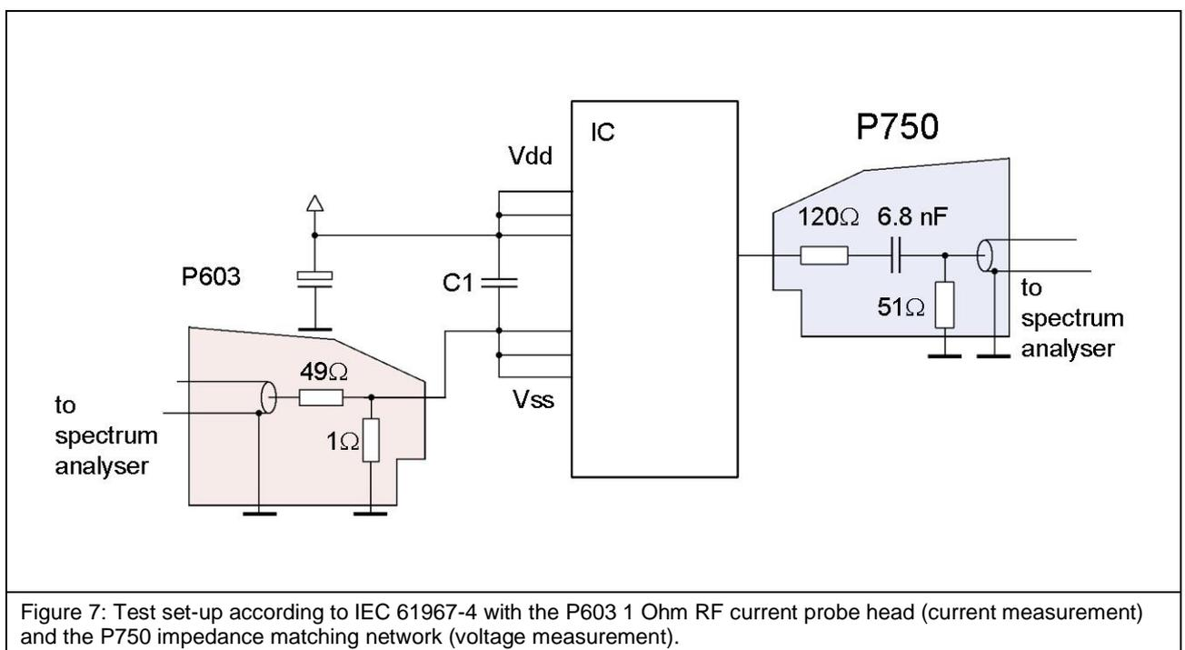
Figure 7: Test set-up according to IEC 61967-4 with the P603 1 Ohm RF current probe head (current measurement) and the P750 impedance matching network (voltage measurement).
