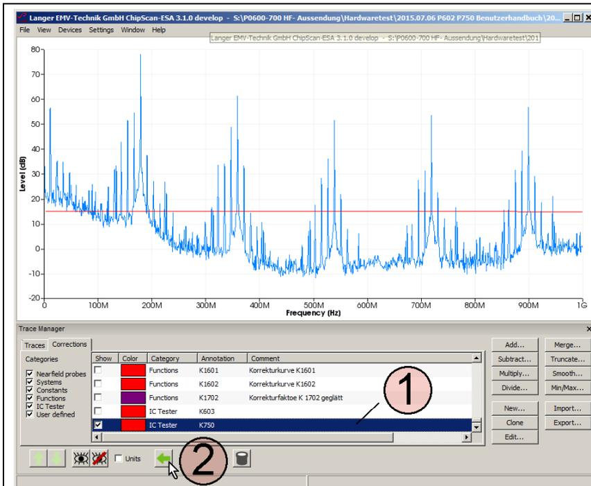
Figure 46: Correction after the measurement; copying K750 from the "Corrections" list to the "Traces" list
