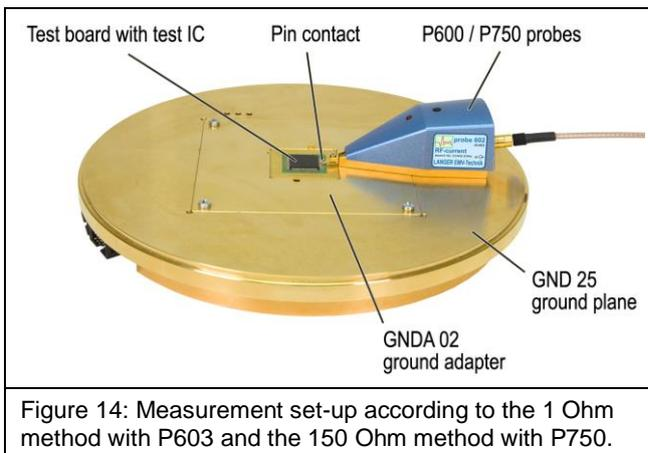
Figure 14: Measurement set-up according to the 1 Ohm method with P603 and the 150 Ohm method with P750.
