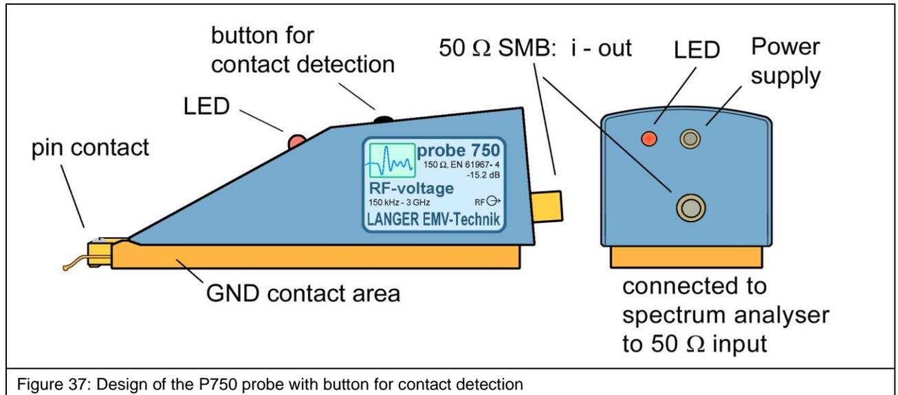
Figure 37: Design of the P750 probe with button for contact detection
