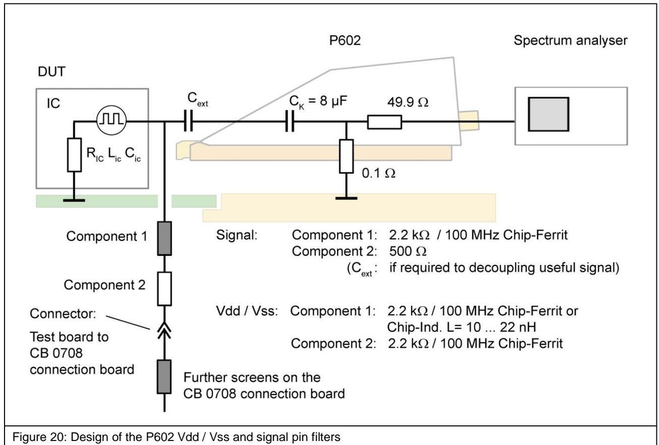
**Figure 20** shows the design of the Vdd / Vss and signal pin filters which are located on the bottom of the test board. Please refer to the "IC test instructions"<sup>1</sup> for a guideline on how to set up a test board.
