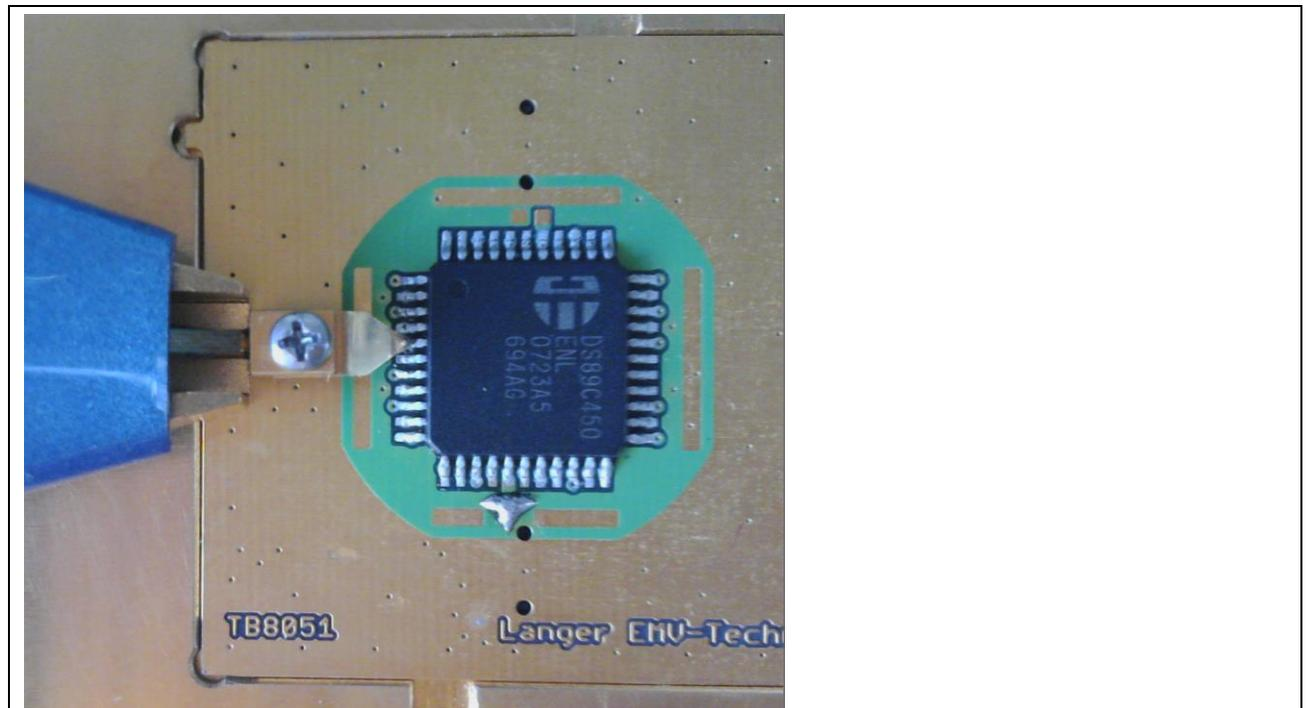
Figure 40: Pin contact visualized with the digital microscope camera.
