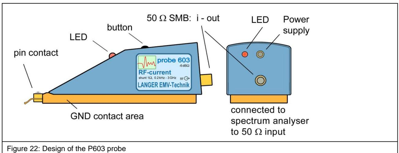
Figure 22: Design of the P603 probe
