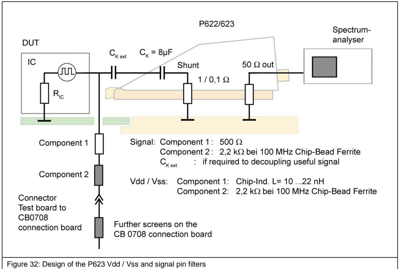
**Figure 32** shows the design of the Vdd / Vss and signal pin filters which are located on the bottom of the test board. Please refer to the "IC test instructions"<sup>1</sup> for a guideline on how to set up a test board.
