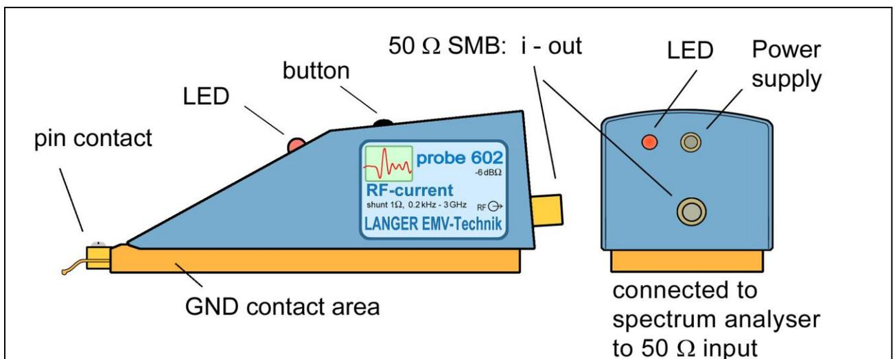
Figure 18: Design of the P602 probe
