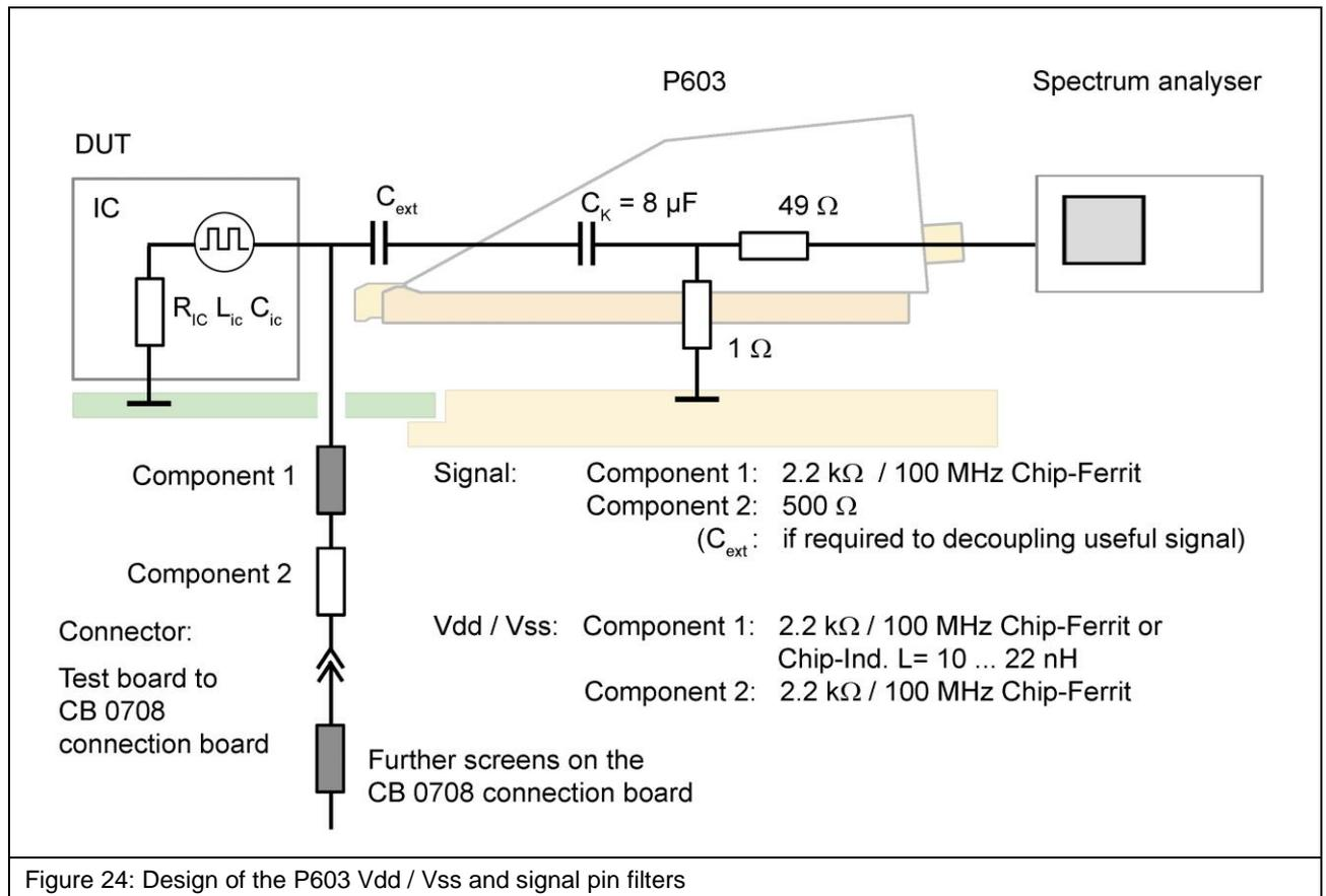
**Figure 24** shows the design of the Vdd / Vss and signal pin filters which are located on the bottom of the test board. Please refer to the "IC test instructions"<sup>1</sup> for a guideline on how to set up a test board.
