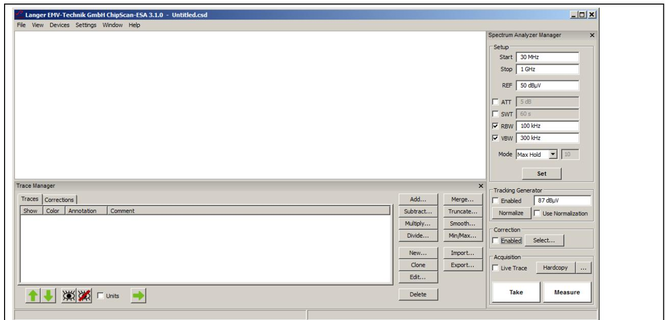
Figure 42: Main settings of the spectrum analyzer in the "Spectrum Analyzer Manager" (right side).
