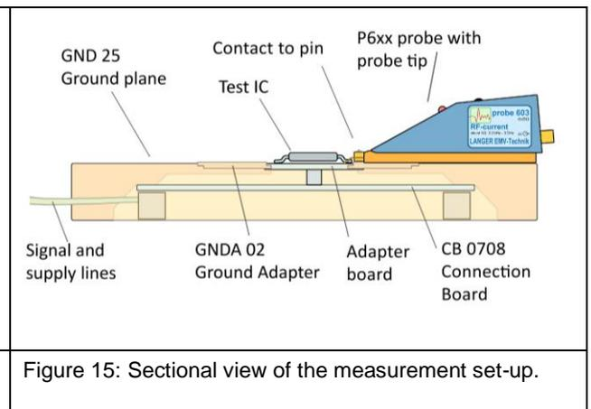
Figure 15: Sectional view of the measurement set-up.
