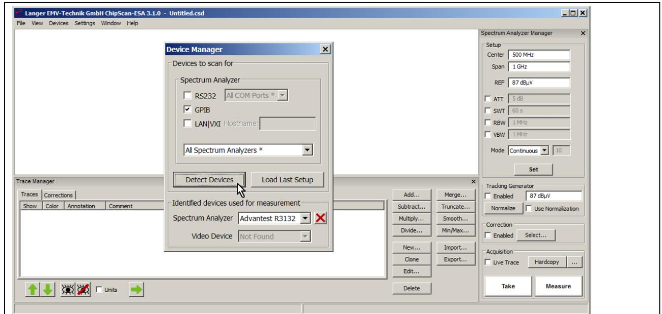
Figure 41: Connecting the spectrum analyzer to the PC.
