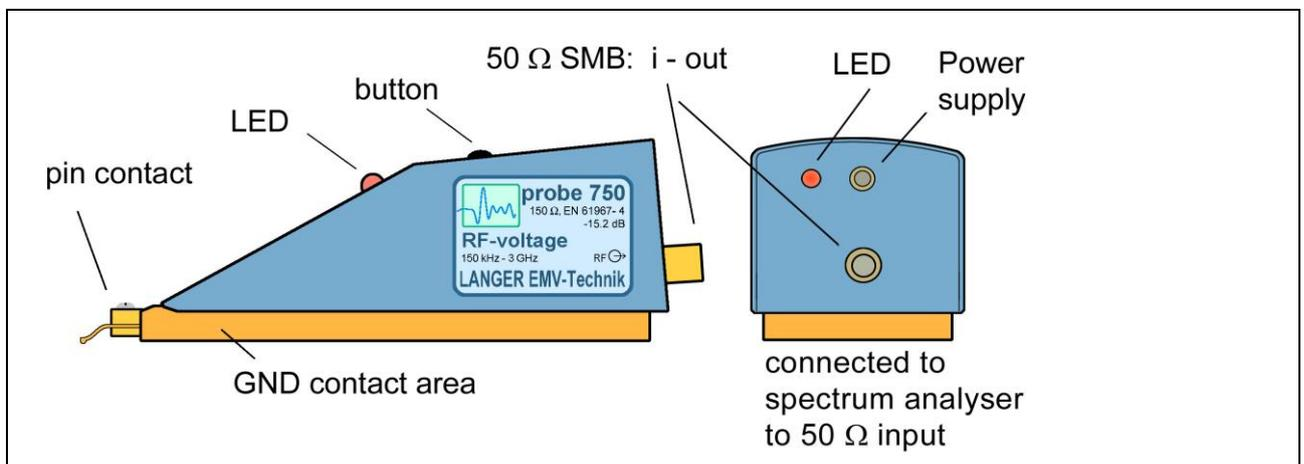
Figure 34: Design of the P750 probe
