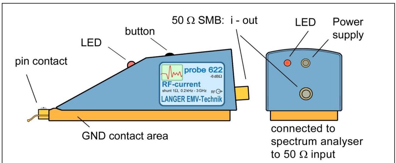
Figure 26: Design of the P622 probe
