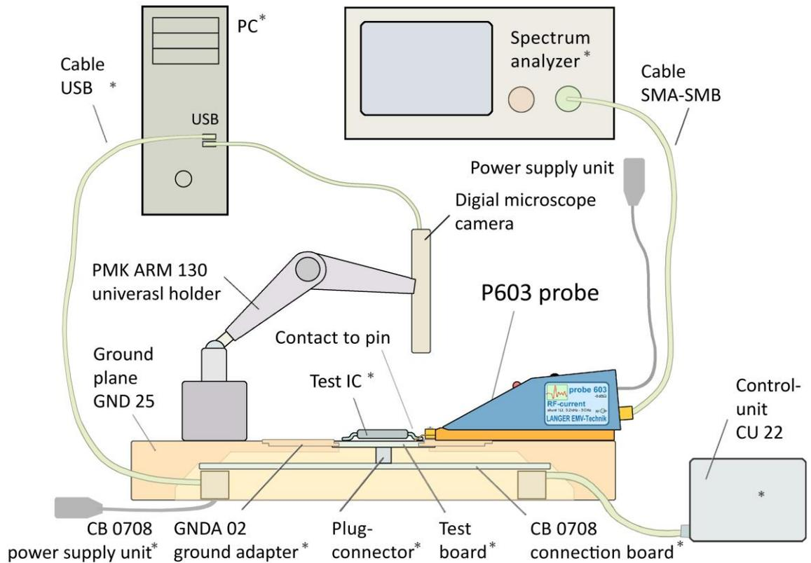
Figure 38: Measurement set-up to measure conducted emissions from integrated circuits (ICs) with the IC test system. Components marked \* are not included in the scope of delivery of the "P603 and P750 RF conducted emissions IEC 61967-4" probe set.
