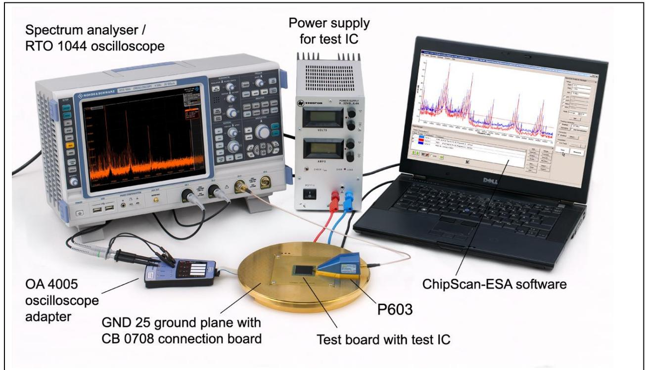
Figure 39: Test set-up with the P603 probe set and ICE1 test environment without a control unit and microscope camera.
