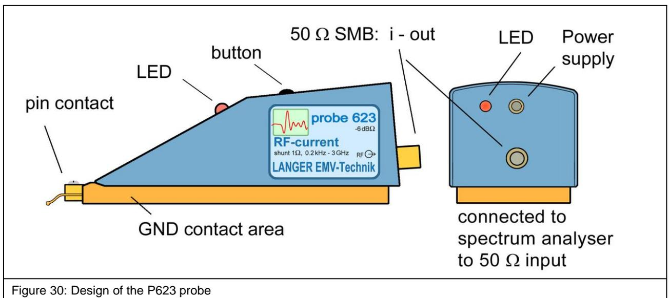
Figure 30: Design of the P623 probe
