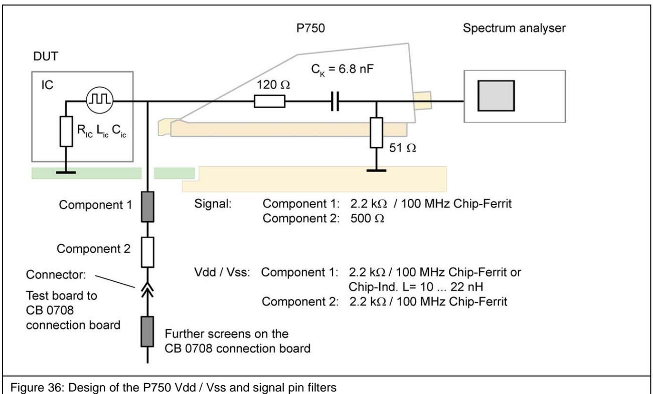
Figure 36: Design of the P750 Vdd / Vss and signal pin filters
